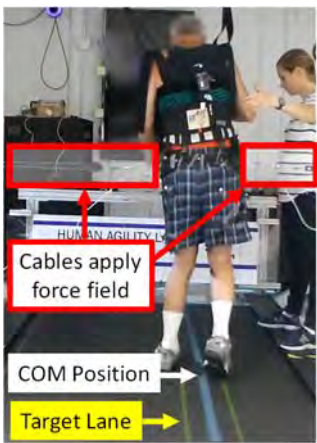
Figure 1: Experimental Setup. During straight walking a cable robot applied lateral forces to a pelvic harness. During all walking mediolateral COM position was projected on the treadmill surface. Participants were instructed to maintain their COM within a dynamic target lane.
