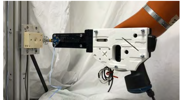
Figure 1: Experimental setup of the KUKA robot retrofitted with a Synthes glenoid reamer and an optical tracker.
