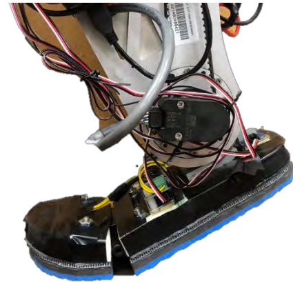
Figure 1: A foot considering a toe joint with spring steel for providing required push-off force. For this study, we constrained the toe joint with a rigid bar such that the stiffness of the foot was infinite. Please see the foot pad was attached to the existing foot of the prosthesis.
