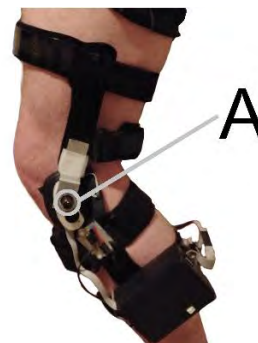
Figure 1: Instrumented knee brace, rotary potentiometer labelled A
