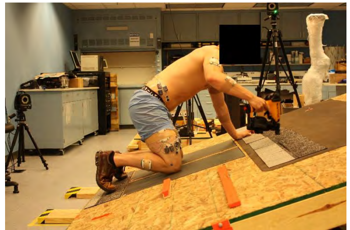
Figure 1: Subject using a nail gun to simulate affixing roof shingles at a 15^\circ pitch.
