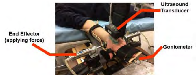
Figure 1. Experimental setup of in vivo ultrasound imaging
