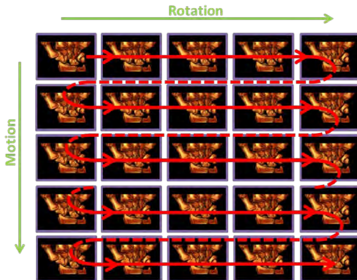
Figure 1 – Generating pre-rendered motion and rotation sequences. After generated a matrix of rendered images, the elements are sequentially formatted into a movie file.
