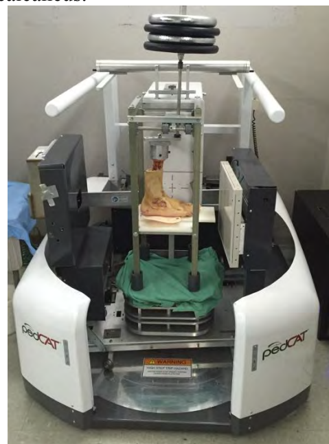
Figure 2: Loaded cadaveric specimen in the weightbearing CT scanner
