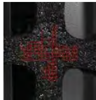
Figure 3: Grids on pig skin sample during biaxial testing.
