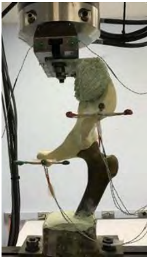
Figure 2: Configuration for axial compression test.
