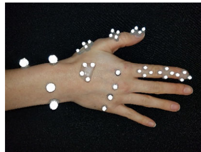
Figure 2: Placement of motion capture targets on hand to capture 3D functional movements.
