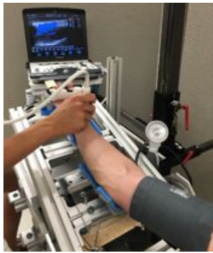
Figure 2: Partial ischemia condition with manual blood pressure cuff placed around upper arm and pressure gauge to monitor compression level.
