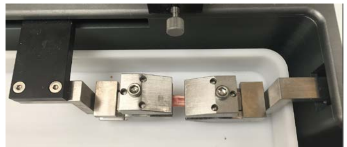
Figure 1: Image of a mounted motion segment; each sample was subjected to 20 phases of cyclic compression/tension.
