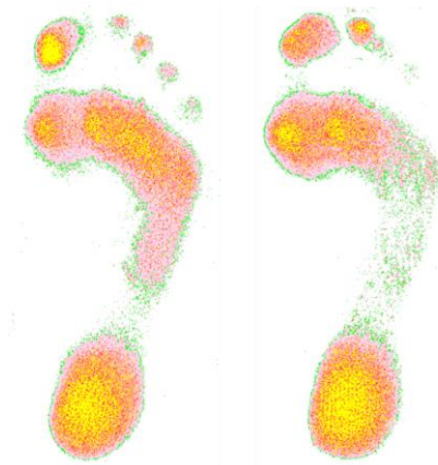
Figure 3: Foot pressure distribution Left side: Normal Socks (NS) Right side: Functional 3D type Socks (3DS)
