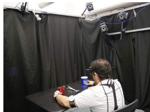
Figure 1: Experimental set-up with motion capture cameras, YCB objects, and subject wearing retro-reflective markers and an eye tracker.
