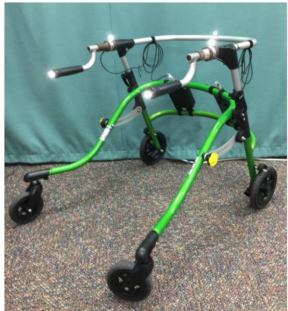
Figure 1: Instrumented walker with five markers (left/right grip, left/right sensor, bar) and load cells at connection from handles to walker.
