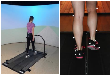
Figure 1. The left picture shows unilateral limb loading with the ankle weight fixed to the left ankle. The picture on the right shows a subject doing the split-belt task.
