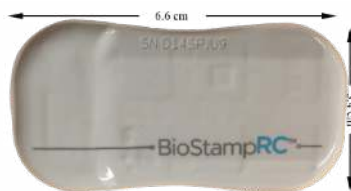
Figure 2: BioStamp wearable sensor is adhered to the skin, and enables direct sensing of human motion and biopotentials (e.g. sEMG, ECG).
