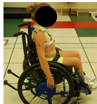
Figure 1: Representative subject in her personal wheelchair with passive markers on her upper extremity and the wheel axle of the SmartWheel.
