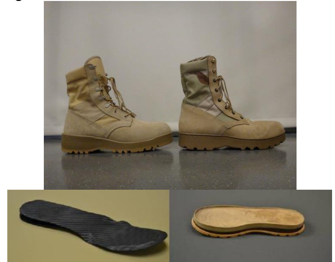
Figure 1: Top: Image of the standard boot (left) and test ESRO boot (right). Bottom: Image of the ESRO (left) and full assembly (right).
