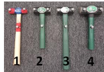
Figure 2: Hammers of varying inertial properties.
