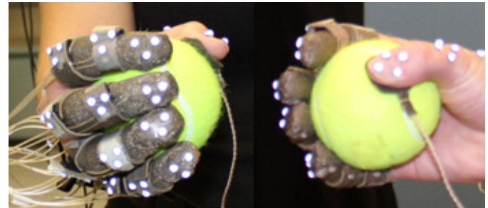
Figure 1. Test setup. The subject grips a tennis ball (65 mm diameter); force sensors are located on the palmar aspects of the finger phalanges.
