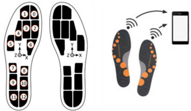
Figure 1. Moticon OpenGo cable-less pressure insoles and their sensor distribution
