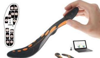
Figure 1. The Moticon OpenGo Insole.
