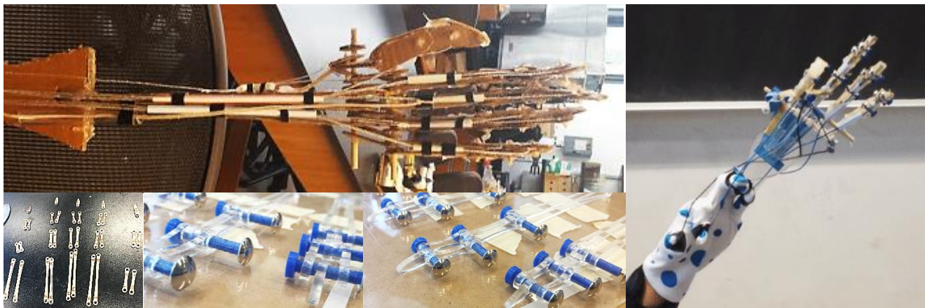
Figure 3: Sample exoskeleton prototyping from using every-day material (upper left) to using laser-cut acrylic and 3D printed parts in final prototype (bottom pictures and right picture).
