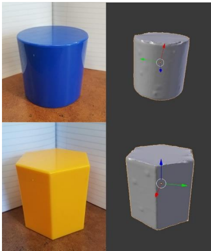
Figure 1: Original picture next to 3D models of the shapes. Bumps on each shape are artifacts left over from adhesive markers the software uses to stitch the image together.
