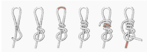
Figure 1: Illustration of three defect locations: Loop, Knot, and Out.
