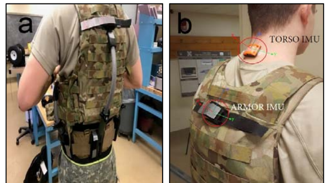
Figure 2a: Load Redistribution Device (ATLAS) and Figure 2b: IMU mounting locations and axes
