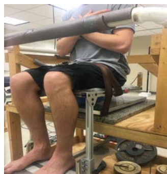
Figure 1: Trunk neuromuscular control testing apparatus. Hemisphere under seat creates instability in the sagittal and frontal planes requiring trunk movement to maintain balance.
