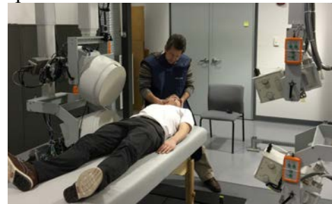
Figure 1: The biplane imaging system configured to collect dynamic biplane radiographs during HVLA manipulation. The X-ray sources are to the right, and image intensifiers and high-speed cameras to the left, providing sagittal-oblique views of the spine without occlusion from the clinician.
