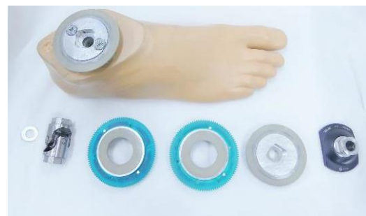
Figure 1: Prosthetic Ankle Parts (left to right): shims, u-joint, two inclined planes with friction pads, top flat plate, and male pyramid
