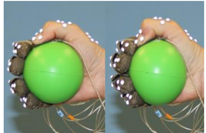
Figure 1. Test set-up. Left: A subject holds a hand rehabilitation ball, with all force sensors being attached. Right: The subject applied the maximal grip force to squeeze the ball.
