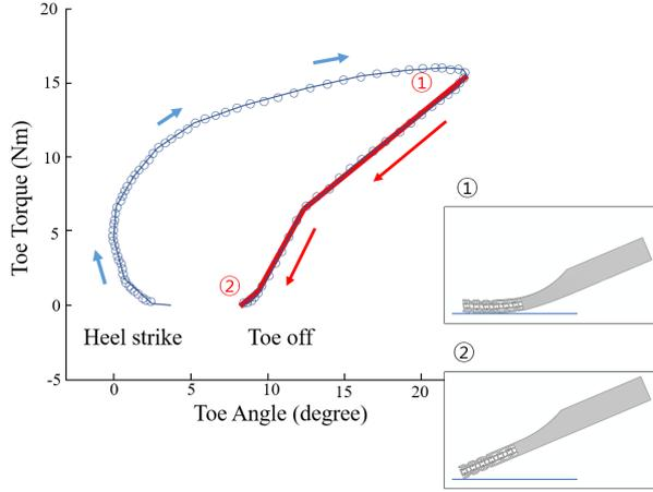
Fig. 1. The toe torque-angle graph of human which shows variable stiffness characteristics [10].
