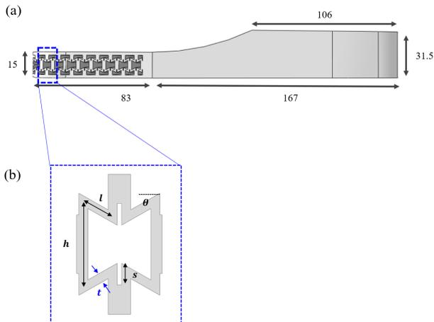
Fig. 2. (a) The dimension of prosthetic foot used in this study and (b) geometrical variables of re-entrant unit cell.
