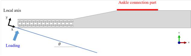
Fig. 4. The boundary condition and loading condition for the FEA of prosthetic foot.
