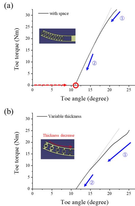
Fig. 8. The toe torque-angle graph as a result of the finite element simulation: (a) for the curved shape foot with bending space; (b) for the designed foot with variable thickness structure.
