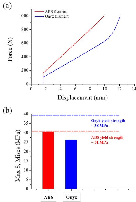
Fig. 6. The FEA results of the re-entrant structure foot with respect to the materials: (a) Force-displacement graph; (b) maximum Von Mises stress.
