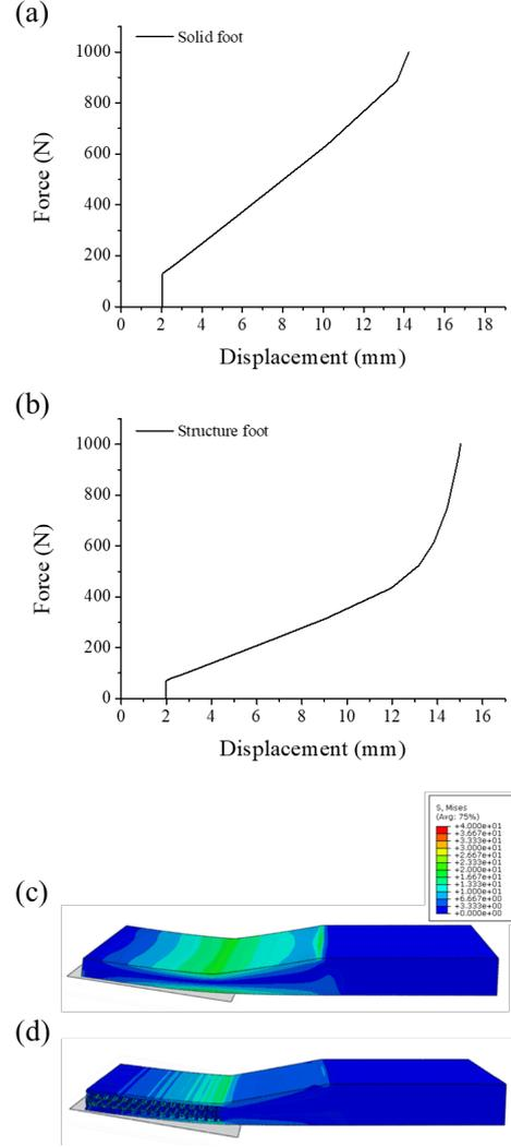
Fig. 5. The force-displacement (FD) curve as a result of FE simulation; (a) solid foot (b) re-entrant structure foot. The stress distribution according to the foot type; (c) solid foot, (d) re-entrant structure foot.
