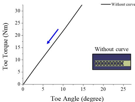
Fig. 7. Toe torque-angle curve as a result of the finite element simulation for re-entrant structure foot.
