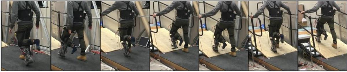
Fig. 10. Prosthesis user walking from flat ground to upslope (<https://youtu.be/Qze2SGNOyUI>).
