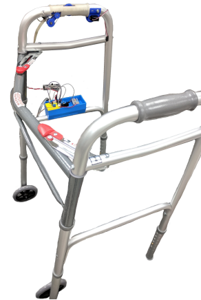
Fig. 1. A standard front-wheel walker with the sensory augmentation system that includes: (i) a skin stretch feedback device embedded into the right handgrip and (ii) a control unit together with the power source packed at the lower part of the walker.
