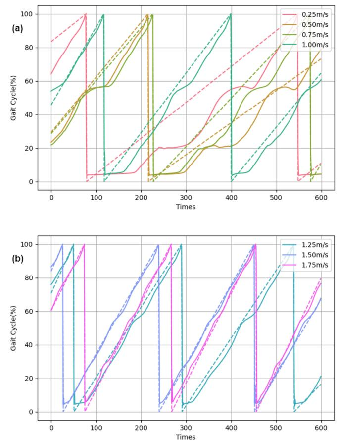
Fig. 4 Gait cycle according to low walking speed (a) and high walking speed (b). Dotted line is ground truth and solid line is predicted cycle.
