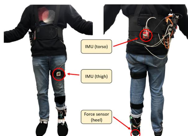
Fig. 2 Wearable sensor set for the gait phase estimation: 2 IMUs for the thigh and torso, and a force sensor for the heel
