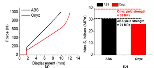
Fig. 6 The FEA results of the first model: re-entrant structure (a) F-D graph; (b) maximum stress
