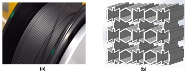
Fig. 3 (a) composite material called “onyx” and (b) auxetic structure (the figure represents combined structure of the re-entrant and honeycomb)
