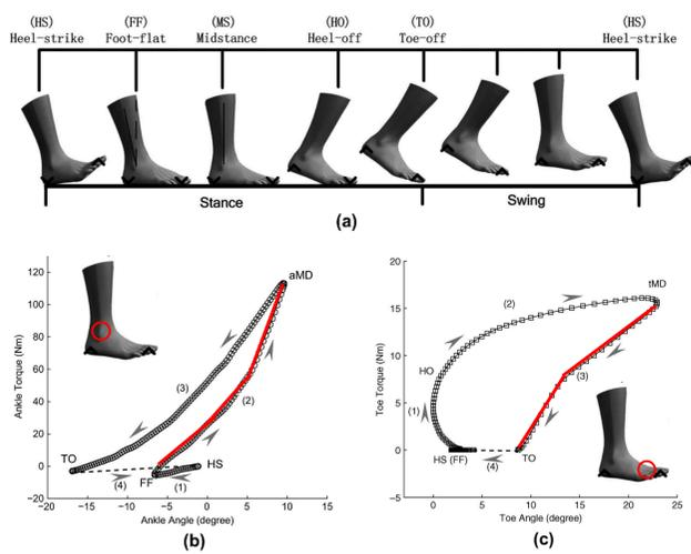
Fig. 1 (a) The schematic of the human gait cycle and the stiffness characteristics (slope of torque-angle graph) of the (b) ankle and (c) toe.
