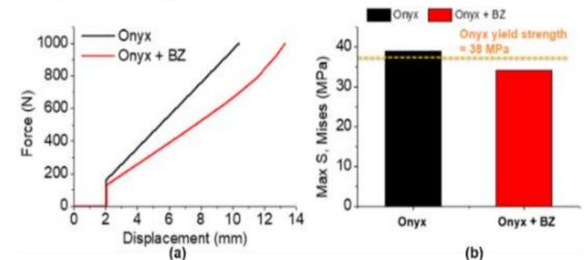
Fig. 7 The FEA results of the second model: re-entrant honeycomb structure (a) F-D graph; (b) maximum stress
