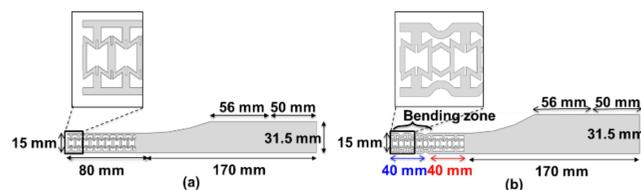
Fig. 4 FEA models. (a) The re-entrant structure was applied in the forefoot; (b) the combined structure of the re-entrant, honeycomb, and BZ was applied in the forefoot
