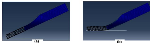
Fig. 5 Toe bending simulation; (a) initial state of prosthetic foot which represents Heel-off step and (b) final state of prosthetic foot which represents Toe-off step.
