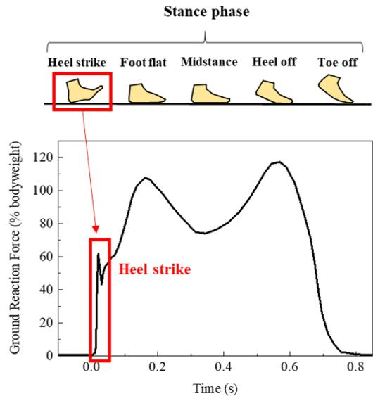
Fig. 1. The gait cycle of human walking and the ground reaction force according to the vertical direction
