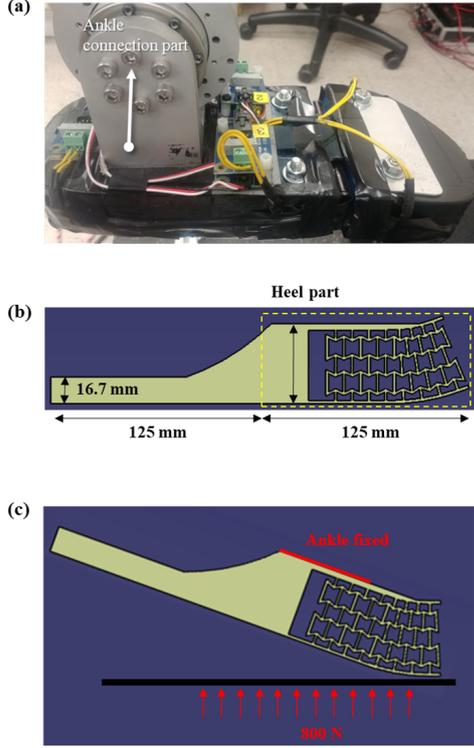
Fig. 2. (a) AMPRO II which was used in the previous study; (b) Overall dimensions of the prosthetic foot; (c) Simulation conditions for the heel strike.
