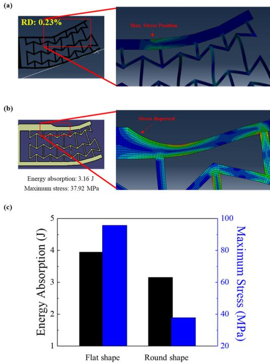
Fig. 6. (a) The stress concentration occurred in the middle part of the upper plate; (b) The FEA results of the structure with and without round shape in the upper plate and (c) the comparison of the energy absorption and maximum stress.
