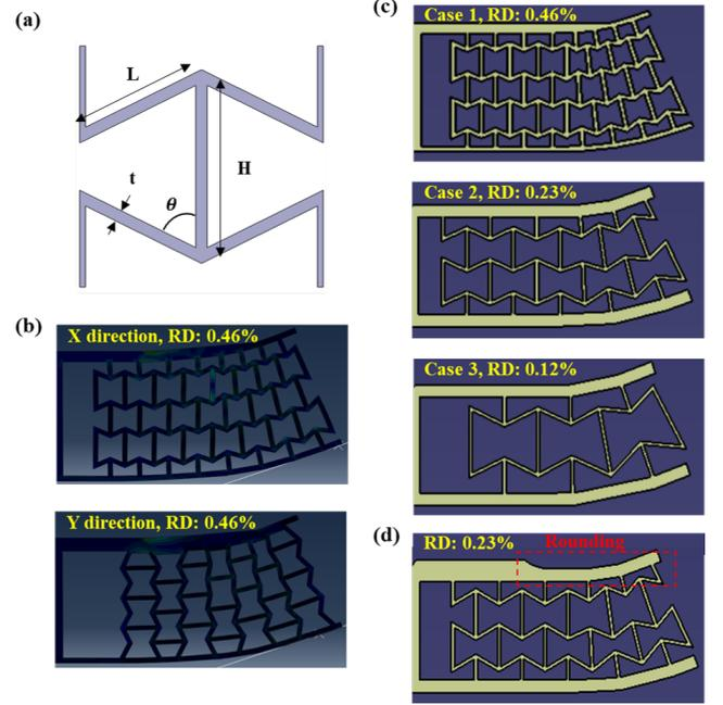
Fig. 3. (a) Geometric parameters of the re-entrant structure unit cell; Heel part design with respect to the, (b) direction of the re-entrant structure and (c) dimensions of the re-entrant structure; (d) Round shape design in the upper plate of the heel part.
