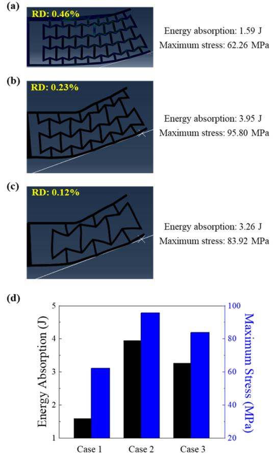
Fig. 5. (a-c) The FEA results of the re-entrant structure with respect to the number of structure and (d) the comparison of the energy absorption and maximum stress.
