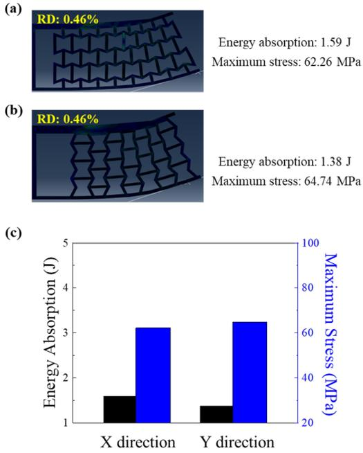
Fig. 4. The FEA results of the re-entrant structure with (a) X direction and (b) Y direction, and (c) the energy absorption and maximum stress.
