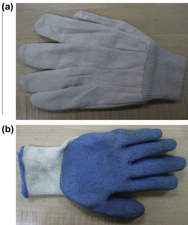
Fig. 2. The polyester glove (a) and latex glove (b) are commonly used at workplaces to protect workers' hand. These gloves can change the coefficient of friction at the hand-handle interface.
