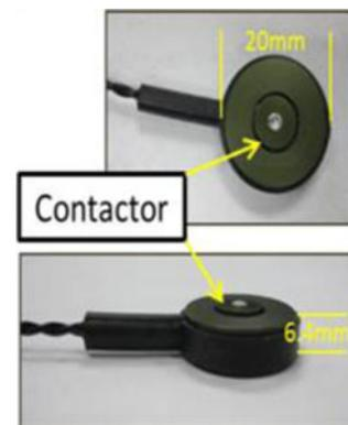
Fig. 3. Vibrotactile device (C-3 Tactor). The contactor is the vibrating part in contact with the skin.
