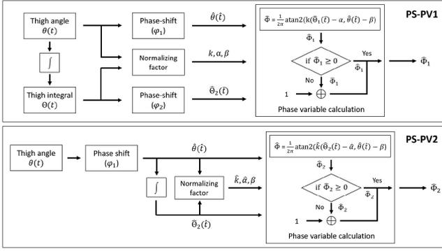
Fig. 6. Overview of phase variable computation using the proposed method. Resulting phase variables are PS-PV1:  $\hat{\Phi}_1(t)$  and PS-PV2:  $\hat{\Phi}_2(t)$
