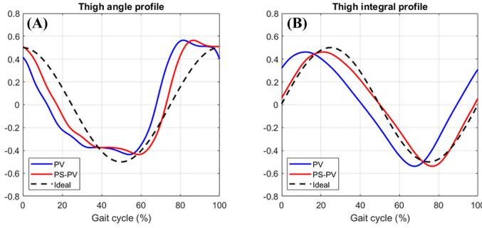
Fig. 2. An example of thigh angle and its integral profile over the gait cycle from a healthy subject. Black dashed lines indicate the ideal sinusoidal functions, while blue and red lines indicate the conventional thigh information and the phase-shifted thigh information, respectively. (A) Two thigh angle profiles (PV vs. PS-PV) and a cosine function, (B) Two thigh integral profiles (PV vs. PS-PV) and a sine function
