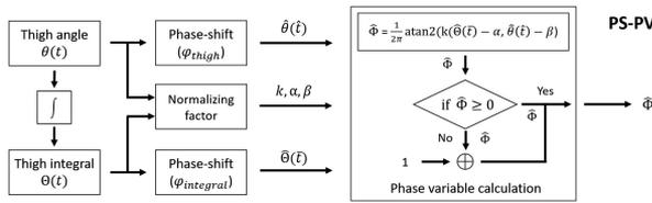
Fig. 3. Overview of phase-shifted phase variable (PS-PV) computation using thigh information. Phase-shifts for thigh ( $\varphi_{thigh}$ ) and its integral ( $\varphi_{integral}$ ) are respectively implemented.
