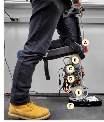
Fig. 7. AMPRO II—a custom-built powered transfemoral prosthesis at Texas A&M University
