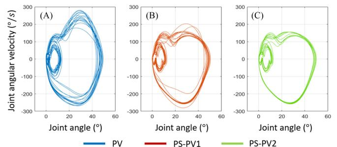
Fig. 11. Phase portrait (joint angle vs. joint velocity) of the knee for 15 consecutive steps (blue: PV, red: PS-PV1, green: PS-PV2)
