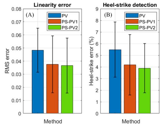
Fig. 9. (A) RMS error between the phase variable and a linear function. (B) Heel-strike detection error (%). (blue: PV, red: PS-PV1, green: PS-PV2). Error bars indicate  $\pm 1$  s.d.
