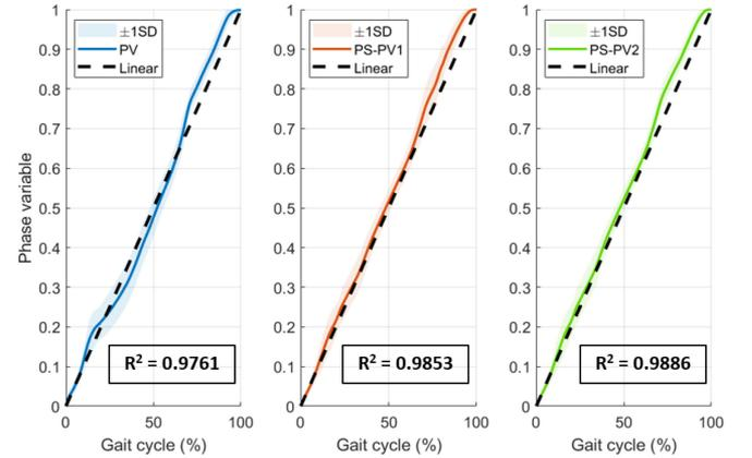
Fig. 8. Resulting phase variable using three different methods (blue: PV, red: PS-PV1, green: PS-PV2). While the solid lines represent the mean of 15 consecutive steps, the shaded regions indicate  $\pm 1$  standard deviation. Black dashed lines indicate the linear function over the gait cycle.
