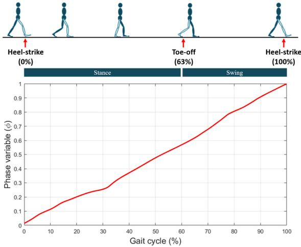
Fig. 1. A gait cycle is usually defined by a heel-strike to another heel-strike on the same leg. A phase variable (y-axis:  $\Phi \in [0,1]$ ) maps the gait cycle (x-axis: 0-100%) to  $[0,1]$ .
