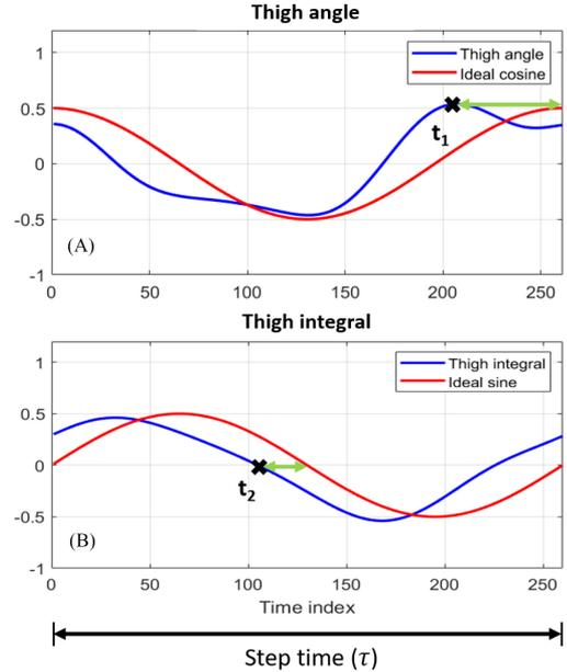
Fig. 5. (A) Phase-shift in thigh angle:  $\varphi_1 = \tau - t_1$ , and (B) Phase-shift in thigh integral:  $\varphi_2 = \tau/2 - t_2$ . Blue lines indicate thigh information, while red lines indicate ideal sinusoids.
