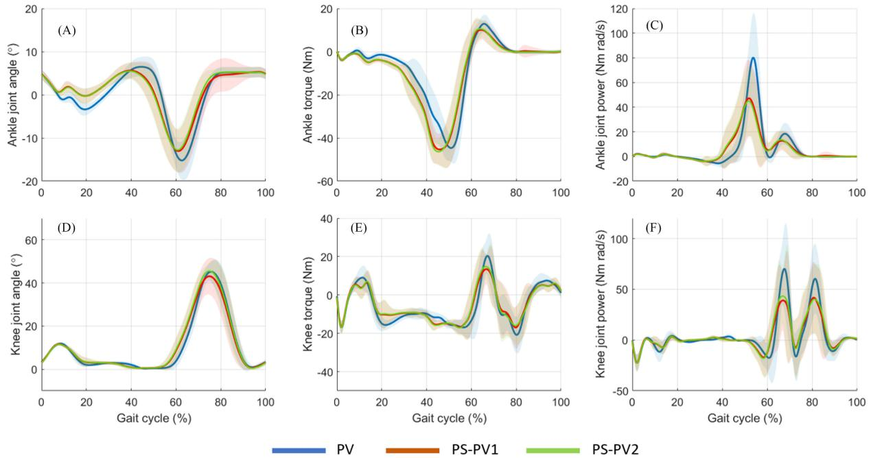
Fig. 10. Joint kinematics/kinetics results (top: ankle, bottom: knee) using the three phase variables: blue: PV, red: PS-PV1, green: PS-PV2. The solid lines and the shaded regions indicate the mean and  $\pm 1$  standard deviation of 15 consecutive steps, respectively.
