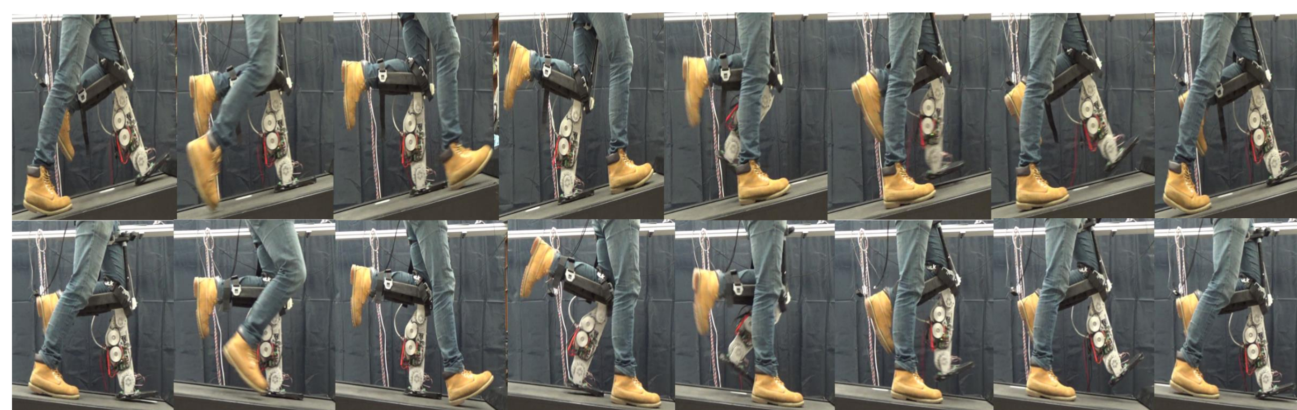
Fig. 6 Prosthesis walking on upslope ( 10^\circ ) and downslope ( -10^\circ ) surfaces
