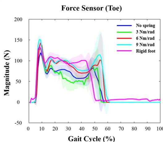
Fig. 4 The toe force profiles during the gait cycle with various toe stiffness conditions. The bold lines and shaded regions are indicated the mean value and the range within one standard deviation. (stiffness1, stiffness2, stiffness3: 3, 6, 9 Nm/rad)
