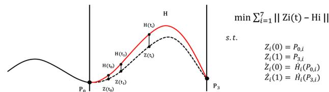
Fig. 3  $H_i$  indicates a human walking trajectory of the  $i^{\text{th}}$  slope condition, where  $i = \{1,2,3,4,5,6,7\} \equiv \{-15^\circ, -10^\circ, -5^\circ, 0^\circ, 5^\circ, 10^\circ, 15^\circ\}$  inclination.  $P_0, P_3$  refer to the joint angle at 60%, 85% of a gait cycle, respectively.
