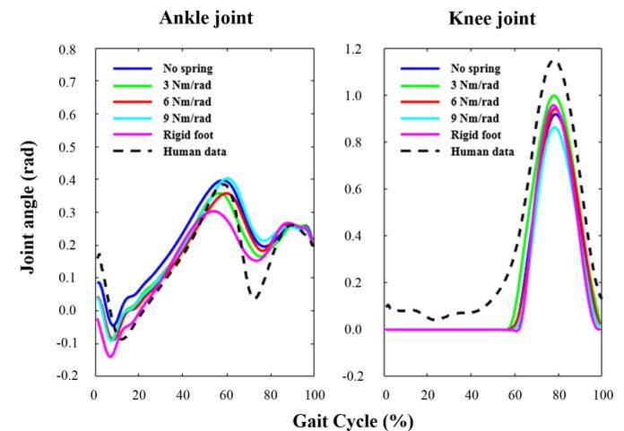
Fig. 5 The ankle (left) and knee (right) joint trajectories of the prosthesis with various toe stiffness. The dashed line is a healthy subject gait.
