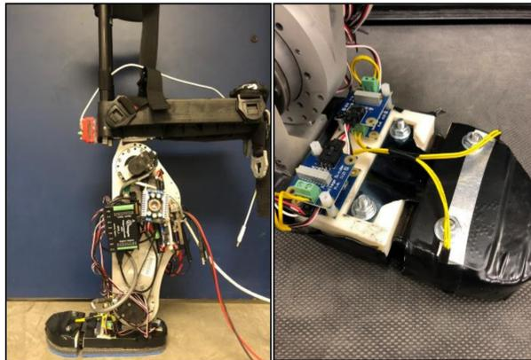
Fig. 1 The powered transfemoral prosthesis AMPRO II (left), and its human-inherent designed foot considering a toe joint with spring steel for providing required PO force (right).
