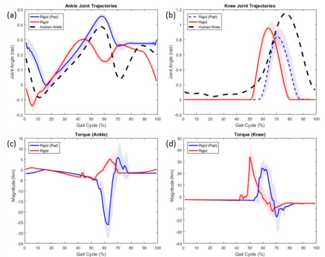
**Figure 3:** Ankle joint trajectory (a), knee joint trajectory (b), ankle torque (c), and knee torque (d) from 2 different cases: rigid foot with a pad vs. rigid foot without the pad. Dashed black line indicates the joint trajectory of the normal healthy gait.
