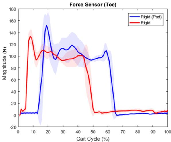
**Figure 2:** Force sensor (toe) data from 2 different cases: rigid foot with a pad vs. rigid foot without the pad. The bold lines are indicated the mean value of the sensor data, and the shaded regions are indicated the range within one standard deviation.
