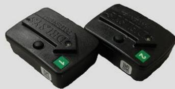
Figure 1: Delsys Trigno IMU sensors used for motion capture system
