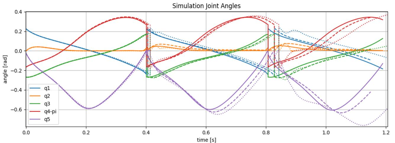
Figure 1. Joint trajectories for three steps (optimal - solid, perturbed *HI* - dashed, perturbed *FL* - dotted)
