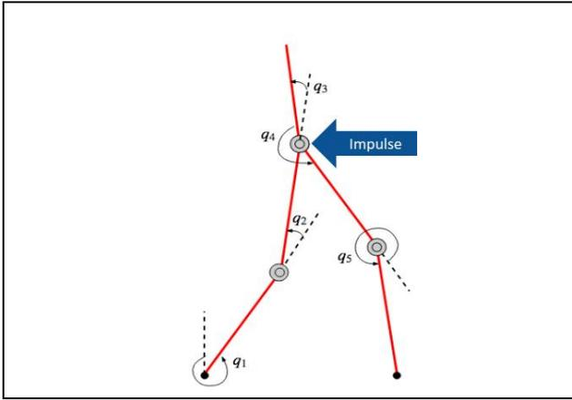
Figure 1. Five-link biped with joint definitions and impulse
