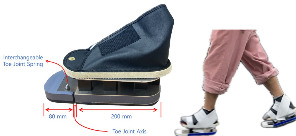
Figure 3. Adjustable toe joint simulation boots.
