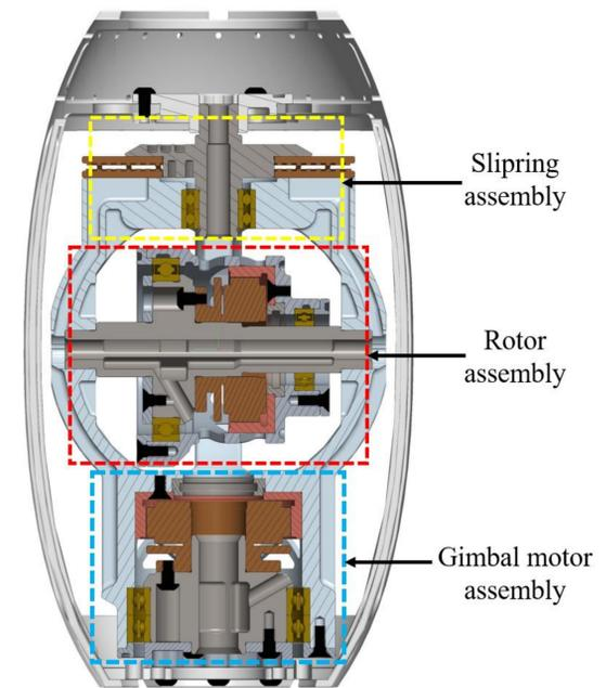
Fig. 3 Main components of HRD
