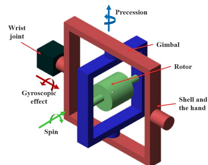
Fig. 1 Device schematic: the red, blue and green components represent the user's hand, gimbal and the rotor, respectively.
