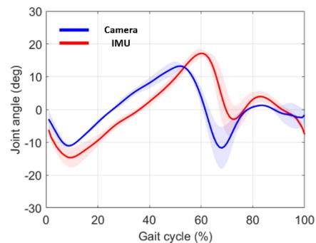
**Figure 2:** Ankle joint angle estimation from two different methods: IMU system (red) and camera-based system (blue). Bold lines and shaded regions refer to the average and  $\pm 1$  s.d. of five consecutive steps, respectively.
